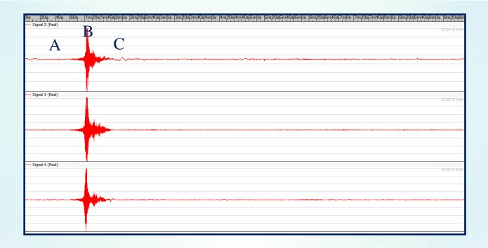
The pressure signals received at the three microphones fall into three regions (A, B, & C).
