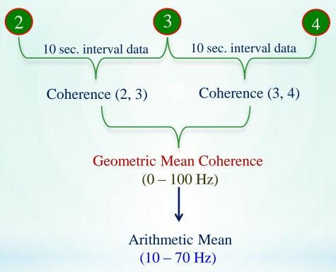
The arithmetic mean of each 10 second interval is used to calculate coherence time history. Then spectrogram is plotted to monitor the life span of wake vortices shed from each aircraft.
