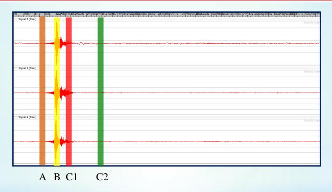
In this slide, the coherence spectrum on takeoff of CRJ is examined in 10-s intervals: prior to burst (brown), at instant of takeoff (burst, yellow), 10-s after takeoff (red), and 50-s after takeoff (Green).
