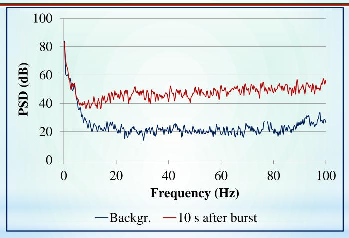
The microphone signals 10-s after takeoff (coherent) are more than 20 dB above the background (incoherent). Since the vortex emission spectrum appears similar to the background spectrum, we concluded that coherence is a better indicator of vortex presence than spectral level. The spectrum is broadband and reveals no features.
