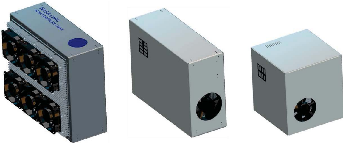
Figure 7 From left to right, original, DAC 1, and DAC 2 designs. The approximate volumes of each are 2,200 cubic inch (original), 1,700 cubic inch (DAC 1), and 1,600 cubic inch (DAC 2).
