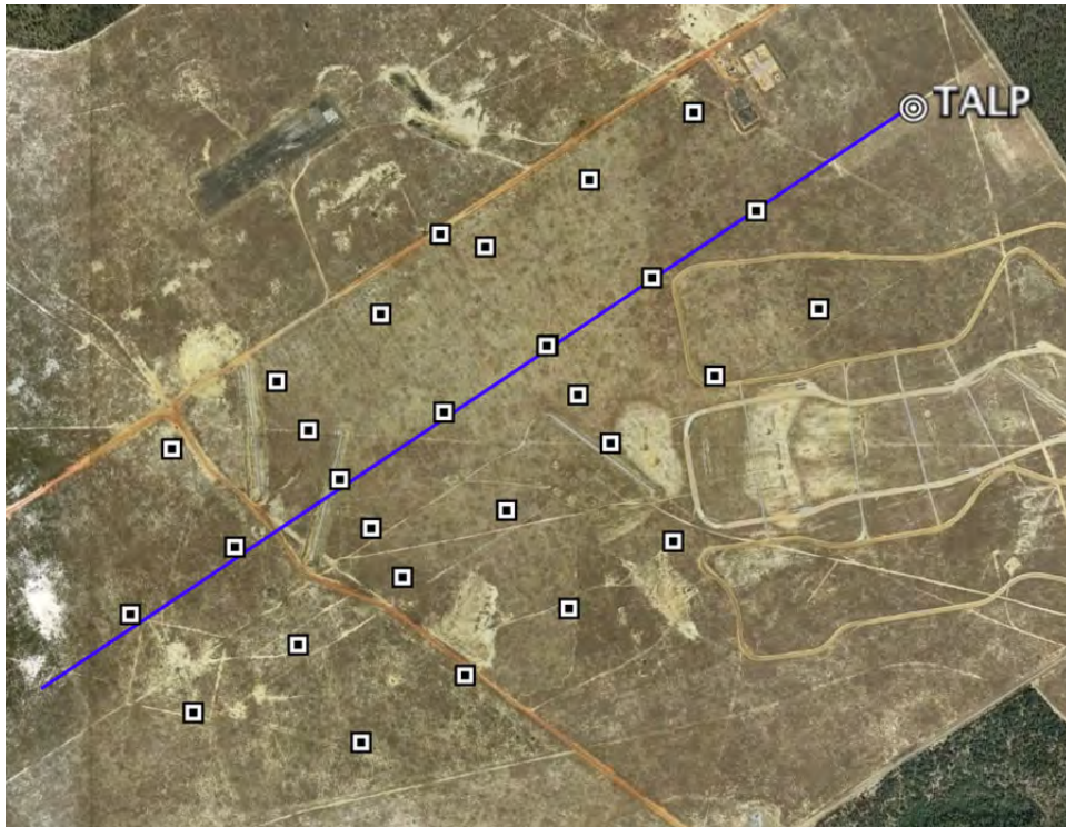
Figure 21: Terminal area microphone array.
