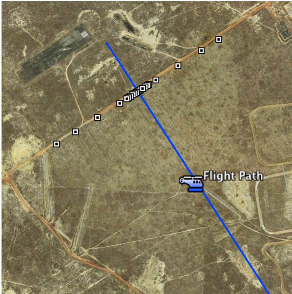
Figure 15: Source noise microphone array.
