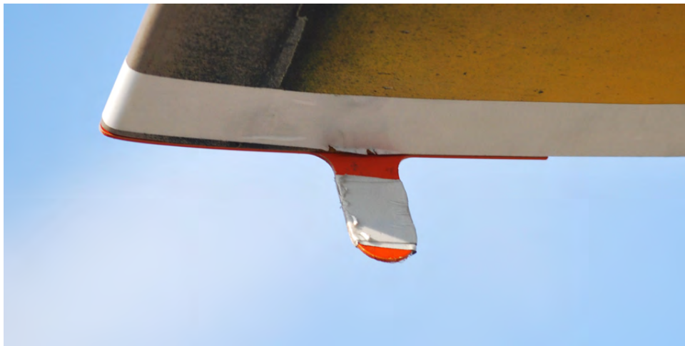
Figure 8: TPP reflective tape mounted on rotor tip.
