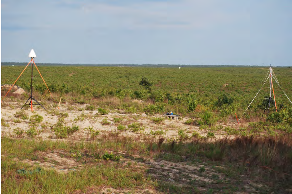
Figure 6: DGPS ground station setup.
