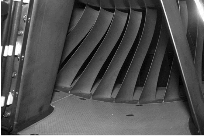
Figure 35.—GE swept and leaned stators tested on CFM-56 engine.
