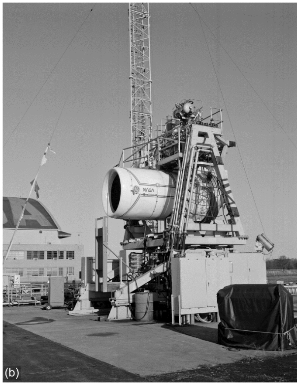
Figure 6.—Outdoor full-scale Quiet, Clean, Short-Haul, Experimental Engine (QCSEE) tests. (a) Microphone array. (b) Engine test stand.
