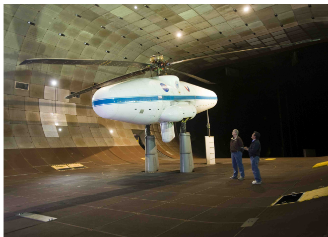
Fig. 1. UH-60A Airloads Rotor mounted on the LRTA in the NFAC 40- by 80-foot Wind Tunnel.
