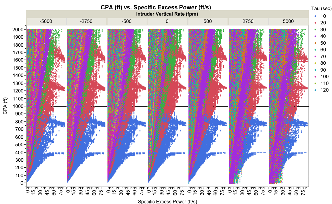
Figure 31: Design Space with CPA Range with only IPD Group; Time-to-go shown by Color; Segregated by Intruder Vertical Rate.
