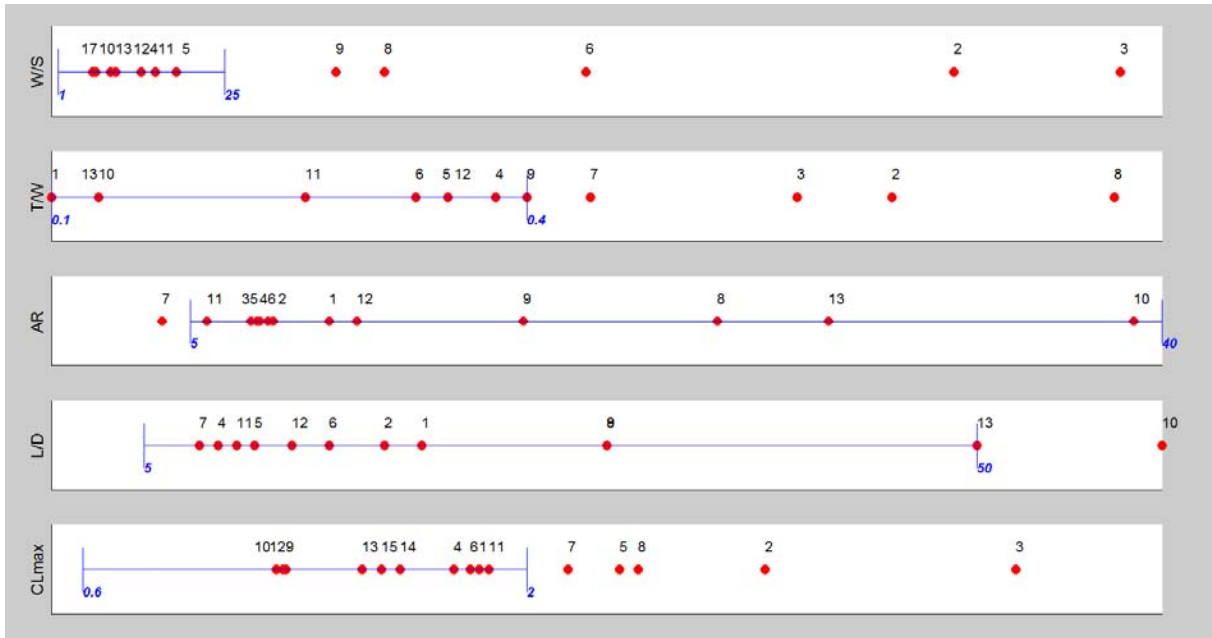
Figure 1: Test matrix of aircraft design parameters. Red dots are the values from the sample aircraft in Table 1 with the number corresponding to the aircraft number in the table. The blue bars show where the test matrix boundaries were set.
