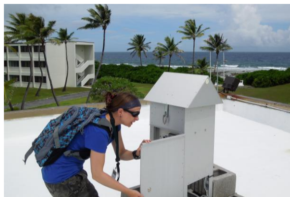
Fig. 1: One of the high volume air samplers installed on Kwajalein Island.
