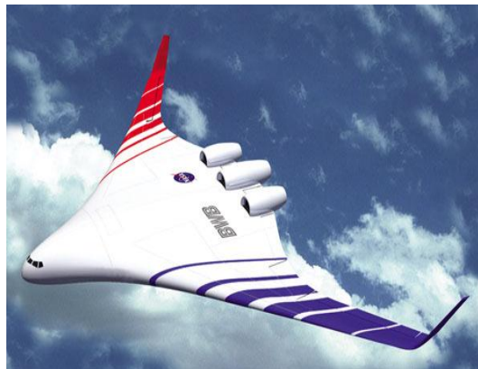
Figure 15: Reference blended wing body aircraft with embedded ultra high bypass ratio turbofan engines.
