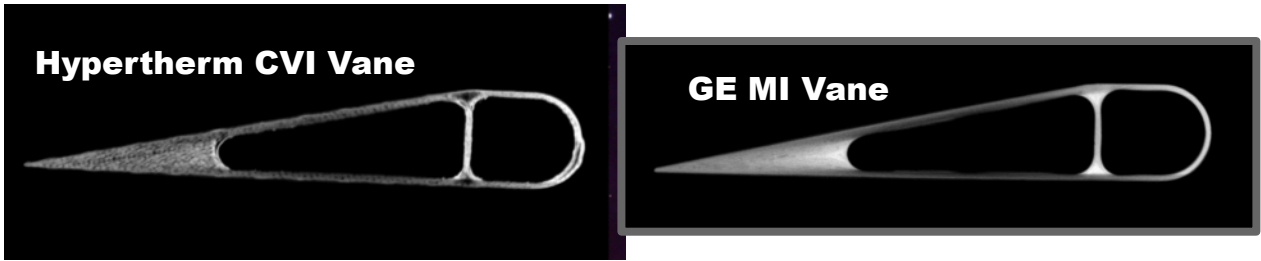
Figure 22: CT images of the Hypertherm CVI & the GE MI vanes. Note the delamination in the Hypertherm vane.
