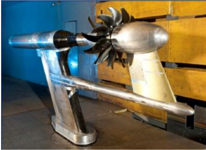
Figure 9: The Open Rotor Propulsion Rig installed in the 9x15 Low Speed wind tunnel on the left and on the right it is installed in the 8x6 Transonic Wind Tunnel in preparation for performance testing at cruise Mach of ~0.8.
