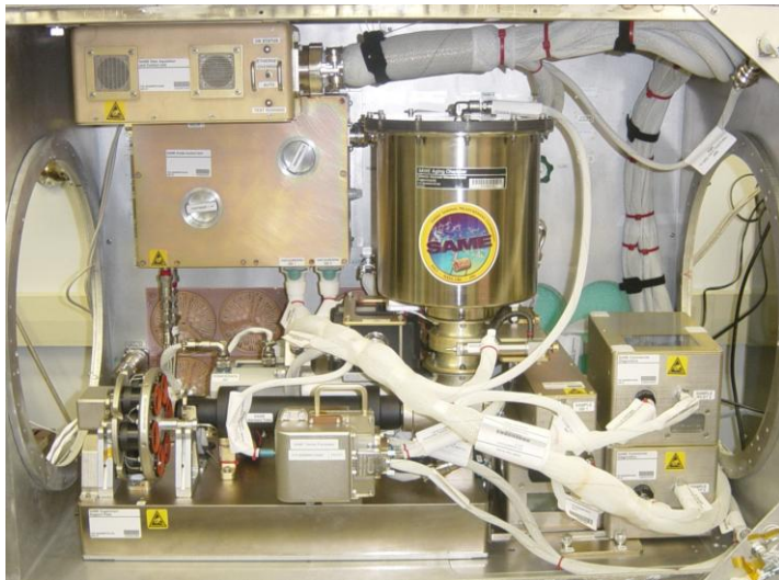
Figure 2b. Photograph of the SAME hardware installed in the Microgravity Science Glovebox on the ISS
