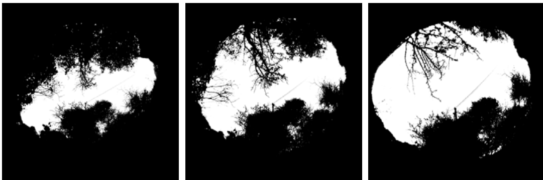
Figure 3. Example of photographic SVFs taken at heights of a) 0 m, b) 1 m and, c) 2m. The associated SVF values are 0.21, 0.34 and 0.50 respectively.
