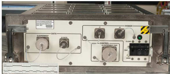
Figure 3. Amine Swingbed Payload: double locker and ISIS drawer control unit before launch.
