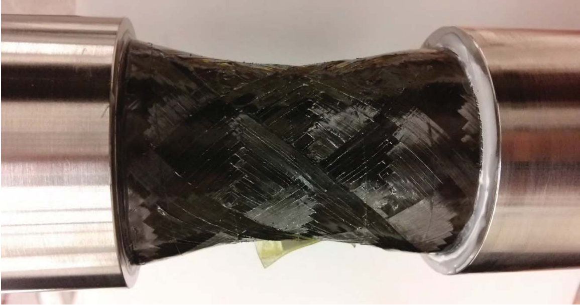
Figure 23.—Failed \pm 45 tension specimen still mounted in test machine.
