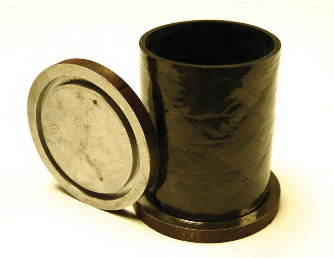
Figure 24.—Compression test end plates and \pm 45 specimen.
