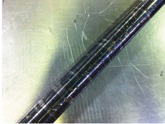
Figure 10.—Photograph of cured hoop-wound tube wrapped in shrink tape.
