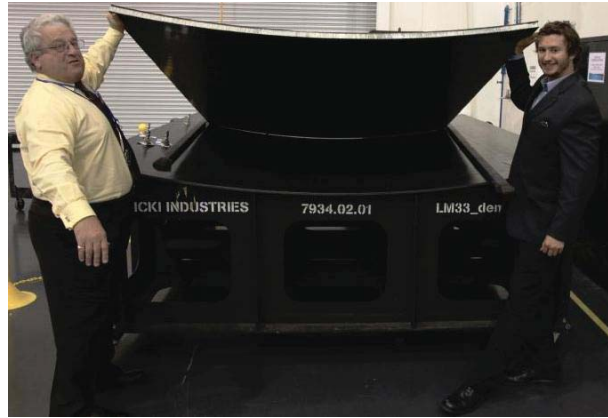
Figure 1. Cured 1/16th arc segment panel and the tool it was molded on.
