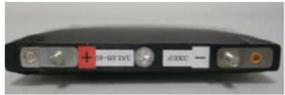
Figure 7. Photo of LIC after the overcharge test showing swelling.
