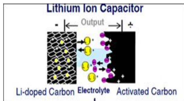
Figure 1. Schematic of Lithium-ion Capacitor (LIC). Courtesy: JSR Micro Inc.
