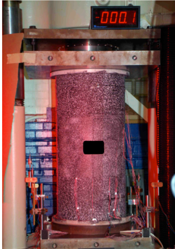
Figure 5. Tow-steered shell with cutout in test stand.
