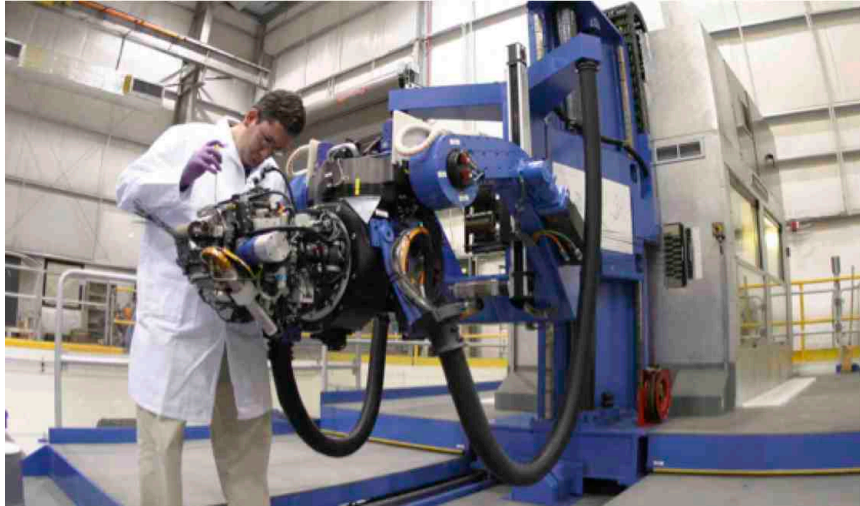
Figure 2. Fiber placement system (Lockheed Martin).
