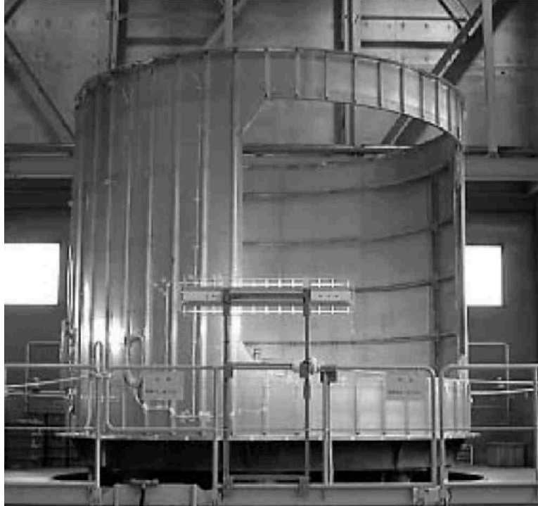
Figure 1. Aerospace structure with a large cutout (JAXA).
