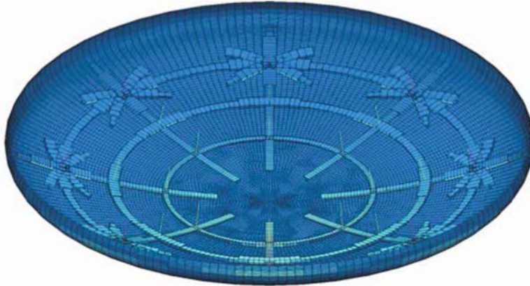
Figure 5. MHSHS model showing the underside frame structure.
