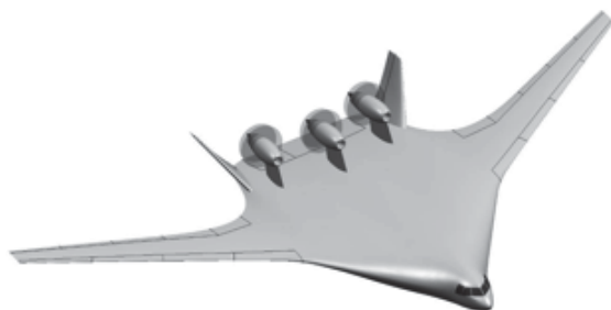
(a) OREIO Hybrid Wing Body aircraft concept with open rotor propulsion system (image credit Boeing 3 ).
