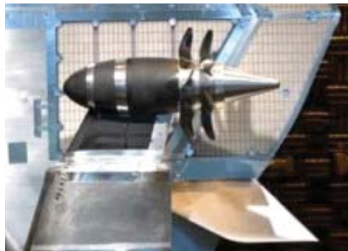
(b) Example F7/A7 open rotor installation with a hybrid wing body airframe from LSAF PAA experiments. 10
