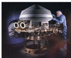
Genesis Sample Return Vehicle stacked on transit stage
