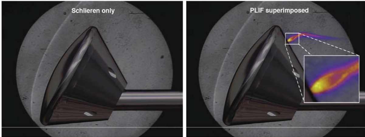
Figure 33. Schlieren and PLIF imaging of Orion RCS from LaRC 31-Inch Mach 10 Air
