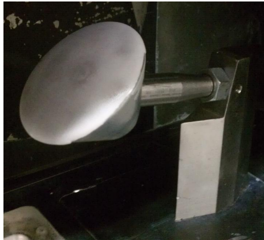
Figure 2: Orion MPCV model at 52° angle of attack configuration with naphthalene heat shield installed in the Mach 5 wind tunnel facility at The University of Texas at Austin.
