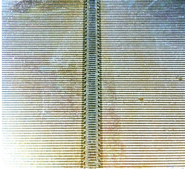
Figure 4. Hot-film array used in checkout of the anemometers used in this study.
