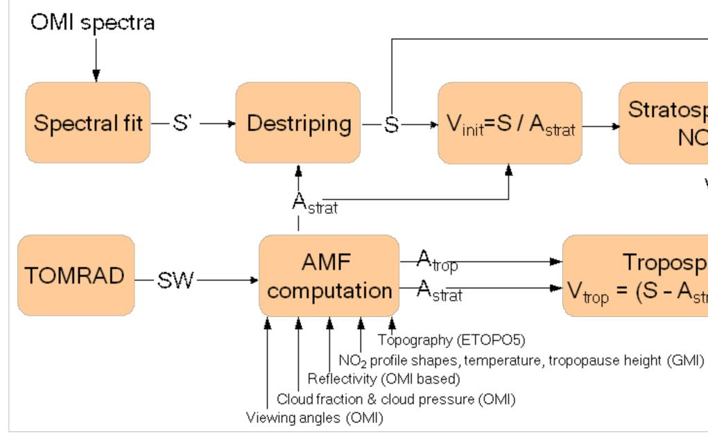
S'  $\rightarrow$  measured slant column density, S  $\rightarrow$  destriped slant column density, SW  $\rightarrow$ scattering weight,  $A_{trop} \rightarrow tropospheric AMF$ ,  $A_{strat} \rightarrow Stratospheric AMF$ .
