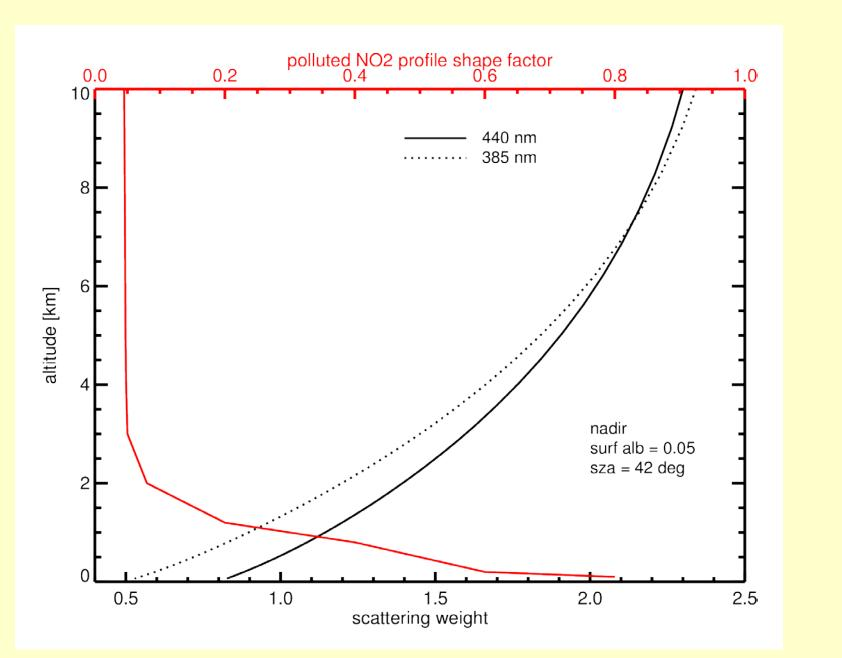
NO<sub>2</sub> vertical profile shape for polluted condition (red line) and scattering weight for a measurement condition (black line) at two wavelengths; 440 nm represents the middle of NO<sub>2</sub> spectral fitting window. Tropospheric AMF derived from the two is critically important for NO<sub>2</sub> vertical column retrievals.
