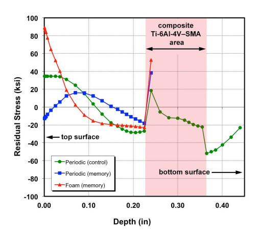
**Figure 5:** Residual stress results from cut compliance testing. The cut progresses from the top surface (on left at 0.00), through the matrix Ti-6Al-4V material (up to 0.22 inch), and then into the Ti-6Al-4V—SMA composite area (denoted by red shaded area).
