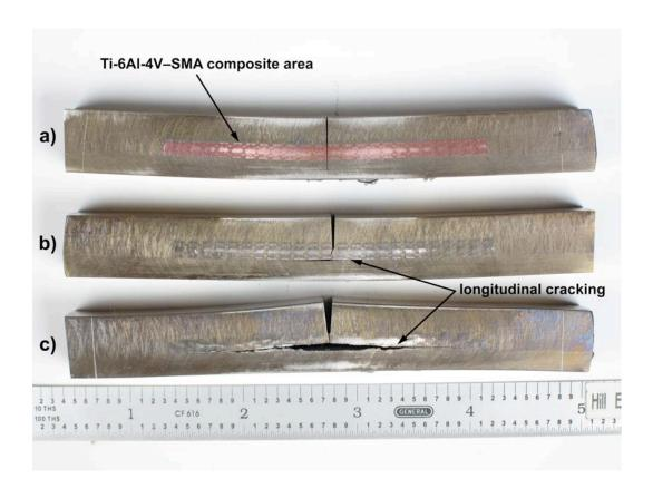
**Figure 4:** Side view photograph of as-tested cut compliance coupons: a) periodic mesh, cold rolled to 4% reduction, no memory activation heat treatment, b) periodic mesh, cold rolled to 4%, memory activation heat treatment, c) foam mesh, cold rolled 4%, memory activation heat treatment. For clarity, the Ti-6Al-4V–SMA composite area is highlighted by the red overlay in sample (a).
