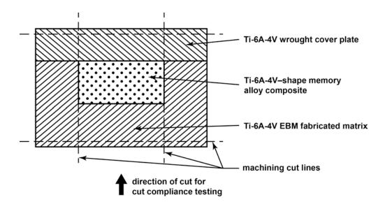
**Figure 3:** Schematic of the cross-section configuration of the coupons. The dashed lines show approximately how much material was machined away in order to prepare the coupons for cut compliance testing. Also note the arrow showing which direction the cut was made with respect to the coupon orientation.
