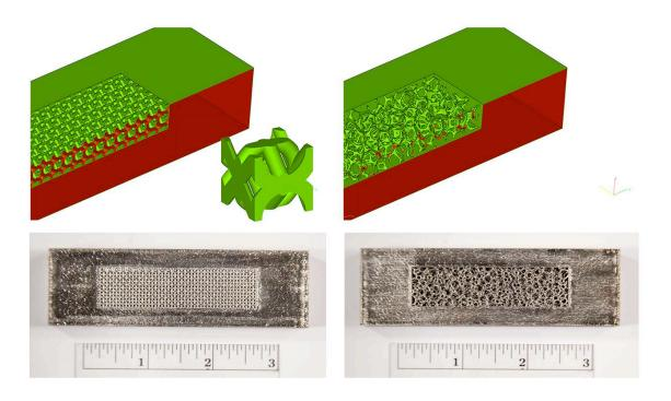
**Figure 1:** Test coupon designs (top) showing section cut through net structure area. Periodic design unit cell shown in inset, upper left. Actual as-fabricated test coupons made via electron beam melting shown on bottom.
