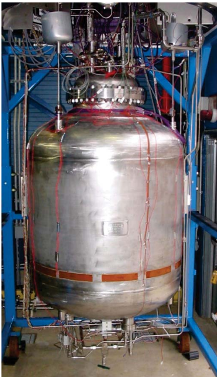
Figure 9.—Test tank prior to installation of multilayer insulation.
