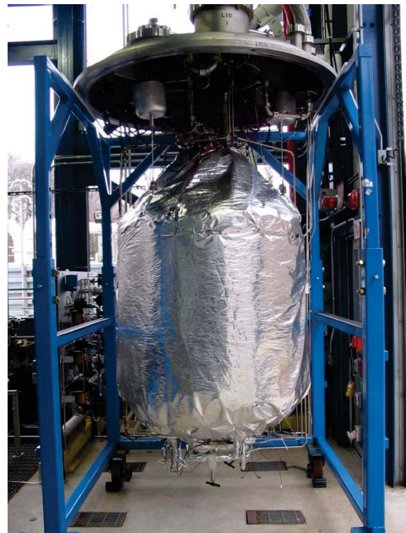
Figure 10.—Test tank with multilayer insulation installed.
