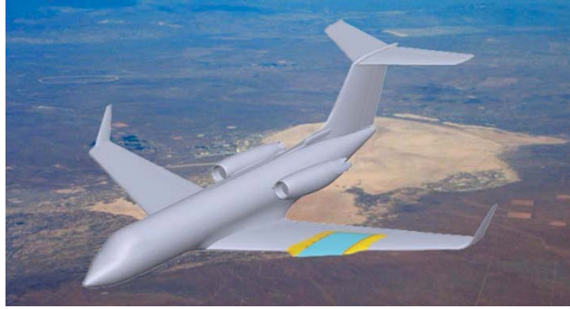
Fig. 2. Conceptual sketch of the SARGE DRE laminar-flow wing glove mounted on the NASA Dryden SCRAT aircraft's left wing.
