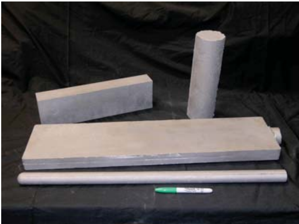
Figure 5 - Cast 60NiTi plate and rod ingots. Forward most cast rod used to produce indentation specimens tested in the present study.
