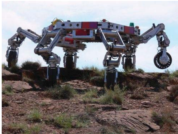
Figure 1: The ATHLETE Rover (NASA Jet Propulsion Laboratory) demonstrating "walking"
