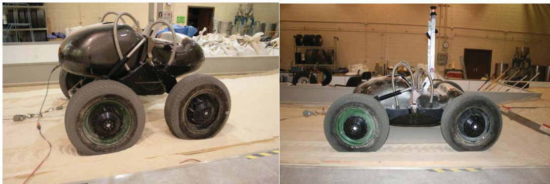
Figure 2: (a) Scarab at high pose (small wheel base), (b) Scarab at low pose (large wheel base)
