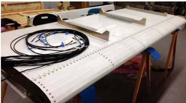
Figure 2. The EcoSAR antennas support single pass interferometry and full polarimetric operation with bandwidths up to 200 MHz.
