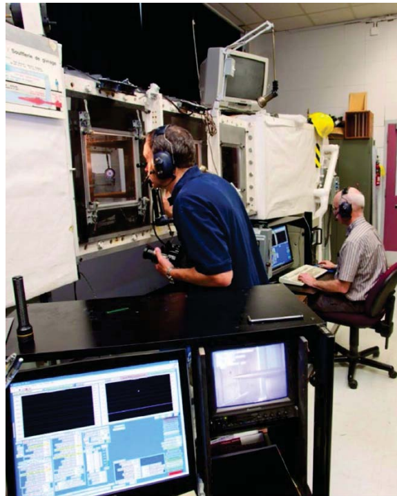
Figure 2.—The AIWT test section with the operator's console in the foreground.
