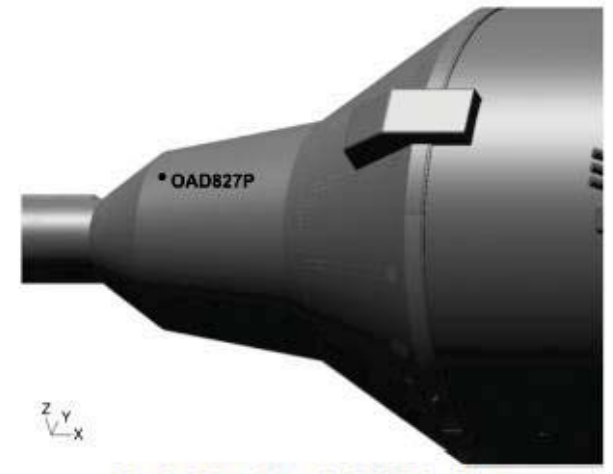
Fig. 9 Transducer OAD827P location.
