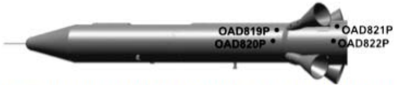
Fig. 6 Transducers OAD819P, OAD920P, OAD921P, and OAD922P locations.
