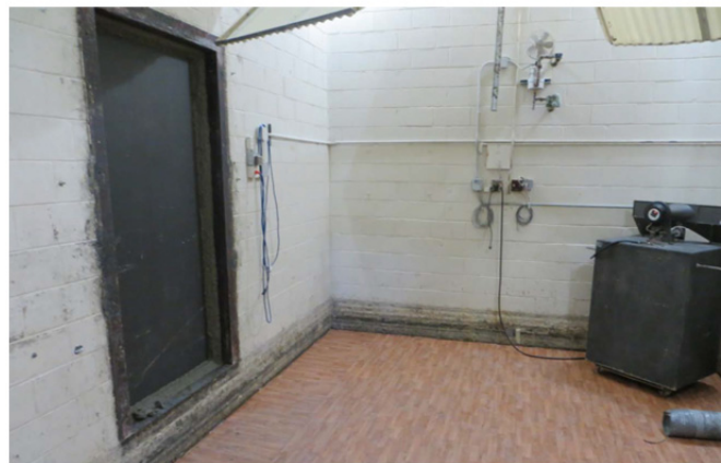
Figure 6.—RAL's TL test setup for TL13-142 (ASTM E-90 airborne sound TL for building partitions and elements method).
