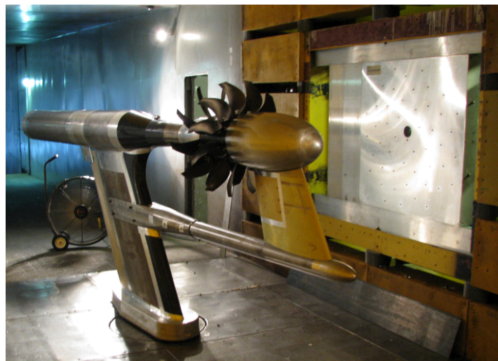
Photo showing Array48 in south wall of Wind Tunnel
