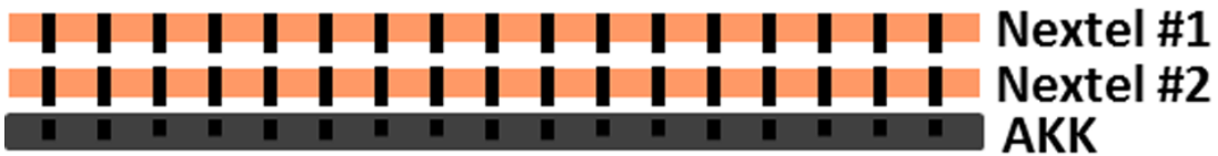
Figure 3: Simplified test article material configuration, consisting of 2 x Nextel 440-BF20 and 1 x AKK.
