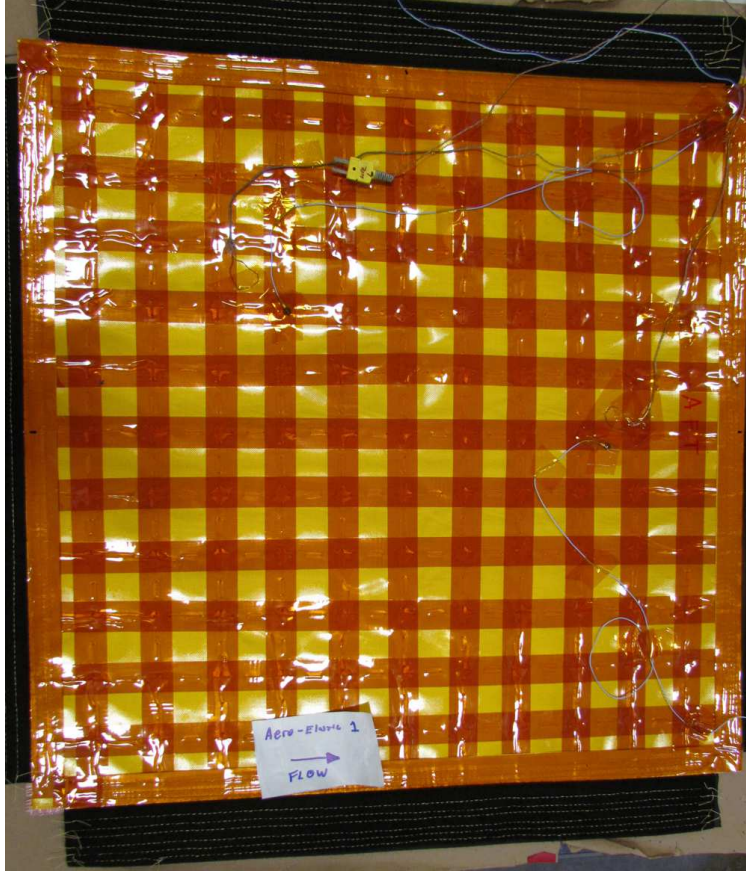
Figure 4: Back side of the simplified test article with attached thermocouple, accelerometer, and Velcro tabs.
