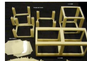
Left: Printed Cubesat structural elements Right: Cubesats deployed from ISS
