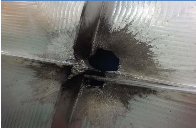
Close-up of simulated MMOD Damage to External ISS Panel
