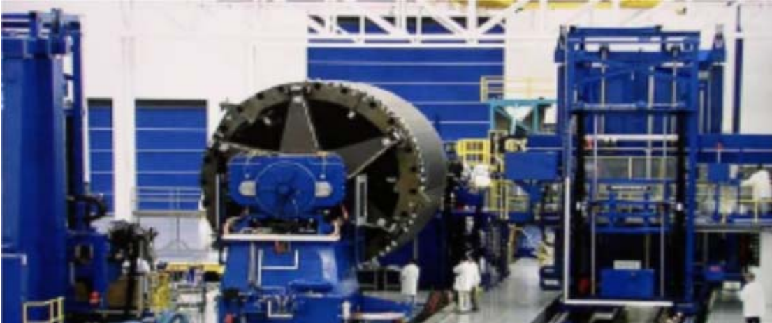
Large Scale Composite Fiber Placement Machine – Composite Cryotanks
