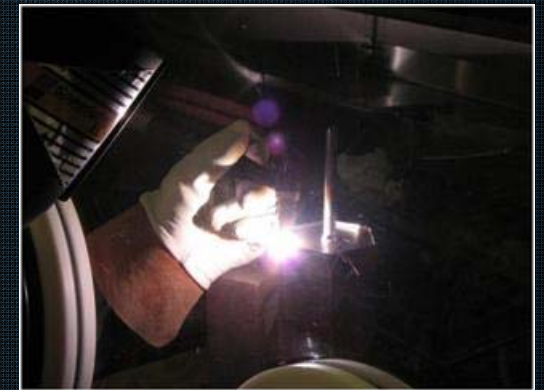
Weld in a argon glove box
