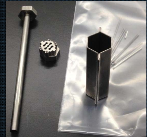
7 Channel Subscale HIP Can
