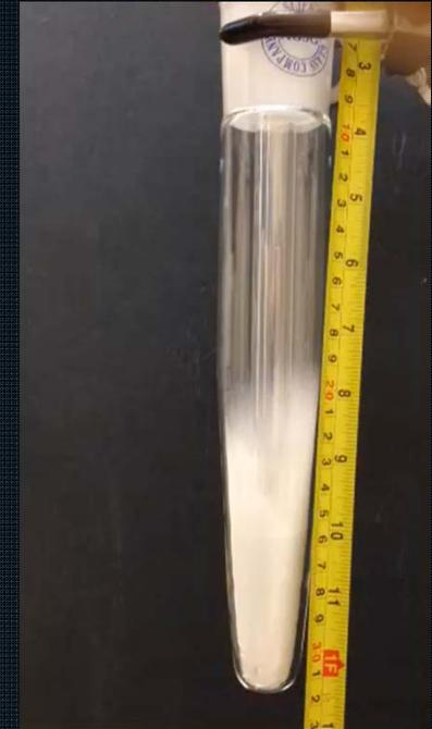
Fluidization: Tapered, 103 g HfO<sub>2</sub>, Ar, 30 L/m outer, 1 L/m inner, flush.
