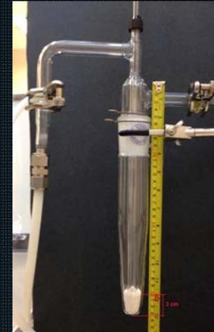
Inverted Reactor Prototype (tapered)
