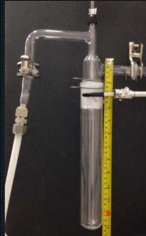
Inverted Reactor Prototype (straight)
