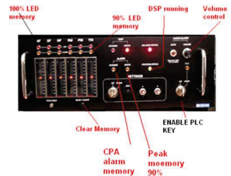
Figure 12. Balance Limit Alarm Monitoring System
