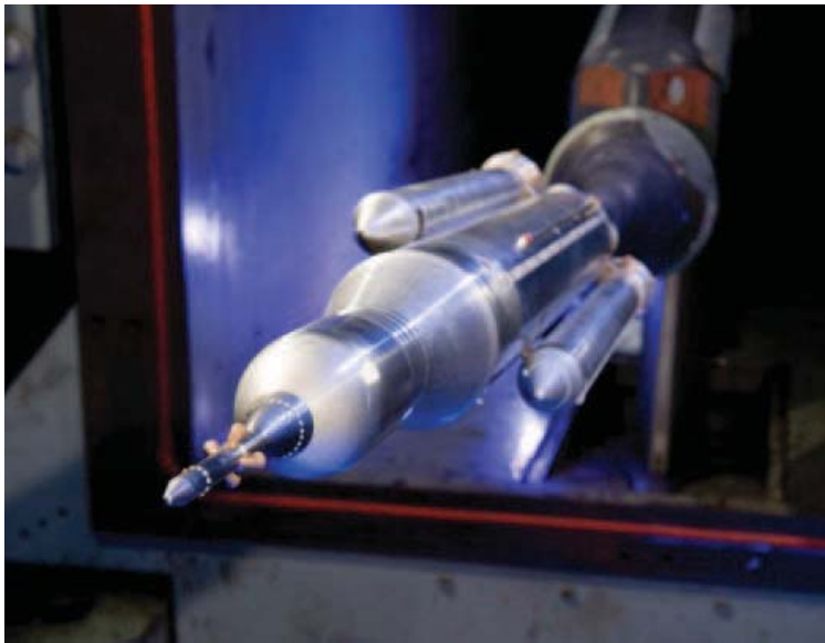
Figure 3. View of the forward portion of the 0.8%-scale SLS-10003 wind tunnel model in the open Boeing PSWT test section. Boundary layer tripping strips are visible.
