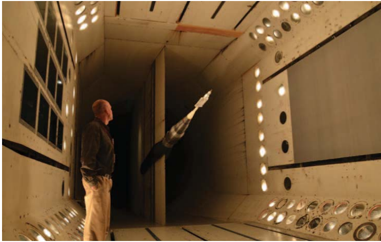
Figure 13. 0.8%-scale SLS model installed in the NASA Langley Transonic Dynamics Tunnel (TDT)
