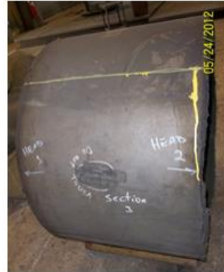
Figure 2-3. Photos of Sectioned Pressure Vessel
