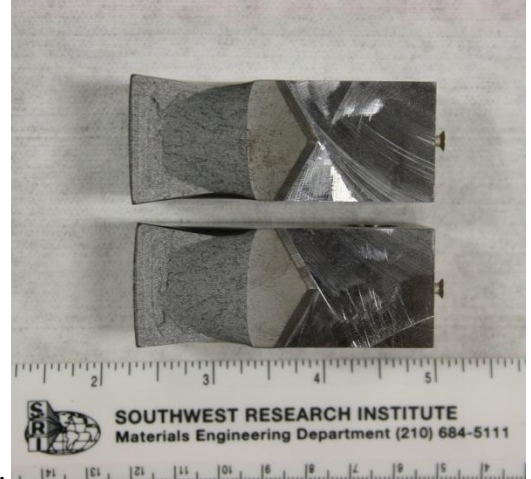
Figure 5-5. Typical A-225 Specimen After Toughness Testing
