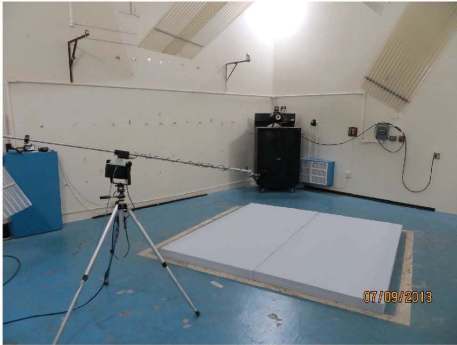
Figure 1 – The test specimen mounted in reverberation chamber.
