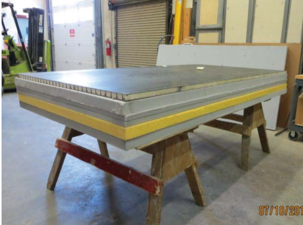
Figure 7.2-5. 8-in.-thick Combination Foam Treatment (TL13-144) (top to bottom layers: FRF panel, 2-in. ML foam, 2-in. ML foam with center mass barrier, 2-in. ML UL foam, 2-in. ML foam)
