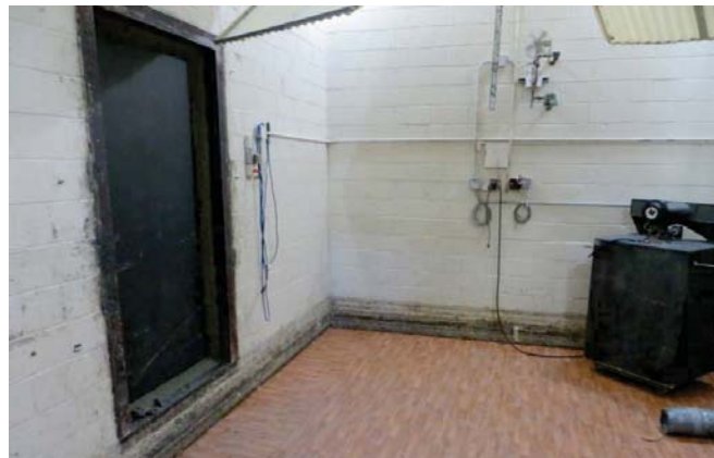
Figure 7.2-2. RAL's TL Test Setup for TL13-142 (ASTM E-90 Airborne Sound TL for Building Partitions and Elements Method)
