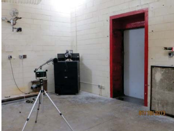
Left, Transmission Loss Receiver Room (4-in. ML foam with mass inclusions shown in test window)
