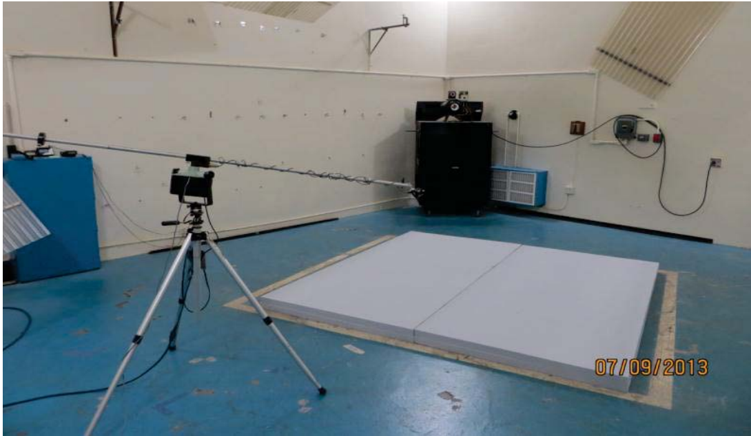
Figure 7.1-2. RAL's Absorption Test Setup (4-in.-thick ML foam, ASTM-C423 Reverberation Room Method)
