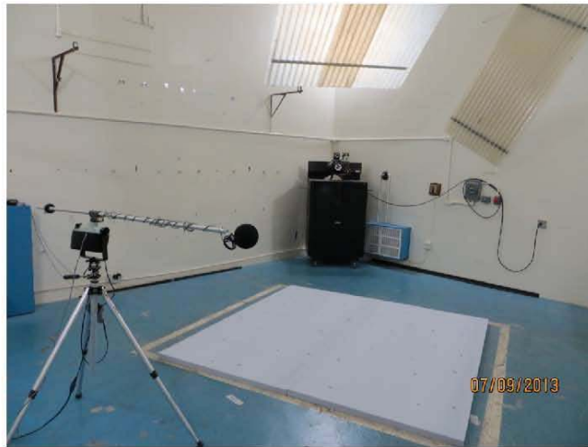
Figure 2 - Test specimen in reverberation room.
