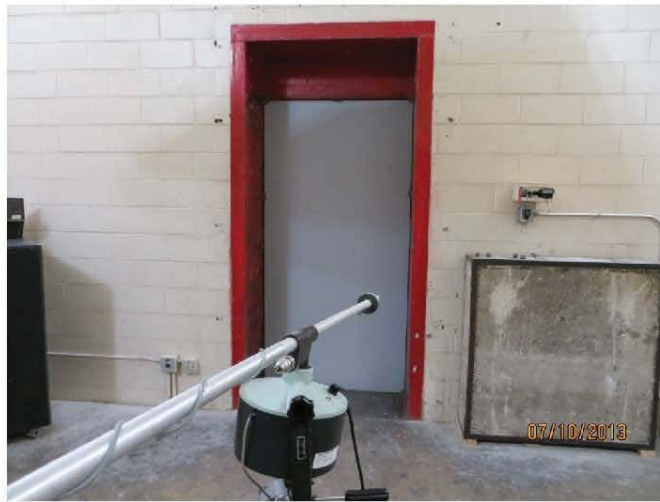
Figure 1 - Receive Room configuration.
