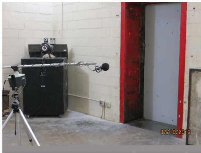
Figure 2 - The Receive Room configuration.
