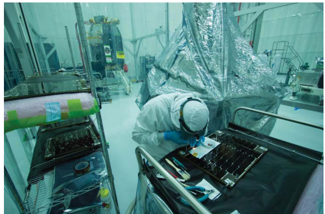
Figure 15: Cell Repair at the Launch Facility
