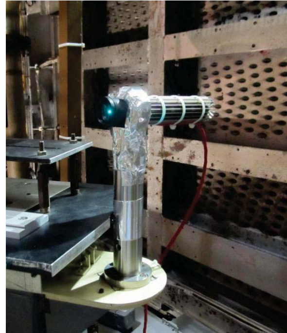
New LED Light Source installed in 8x6
