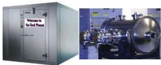
Figure 11 – MAV Solid Propellant Aging Test Chamber
