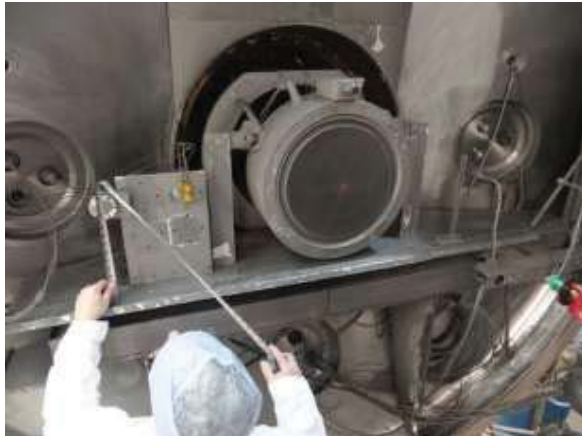
Figure 3 – NEXT LDT Thruster post-test inspection
