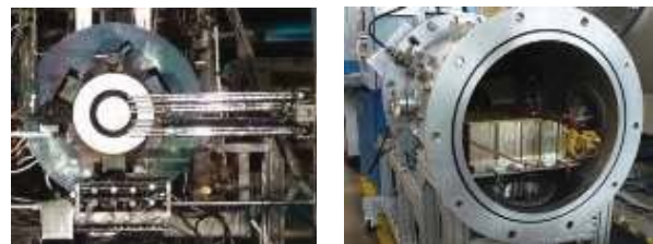
Figure 7 – HIVHAC EDU Thruster and Colorado Power SBIR PPU undergoing performance testing.
