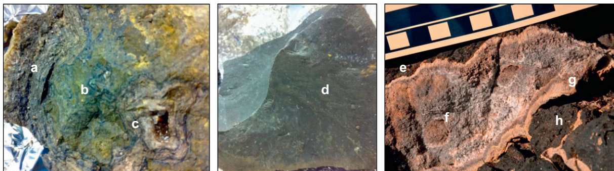
Fig. 4. Left: Knorringfjell sample with (a) black mudstone (AM10-05-BM), (b) green mudstone (AM10-05-GM), and (c) white lithology (AM10-05-WL). Middle: (d) Micrite (AM10-13-M) sample from Knorringfjell. Right: Sigurd fjell sample with (e) external carbonate crust (AM10-27-CS), (f) internal carbonate (AM10-27-CI), (g) carbonate/basalt interface cement (AM10-27-CB), and (h) basalt (AM10-27-B). (For interpretation of the references to color in this figure legend, the reader is referred to the web version of this article.)
