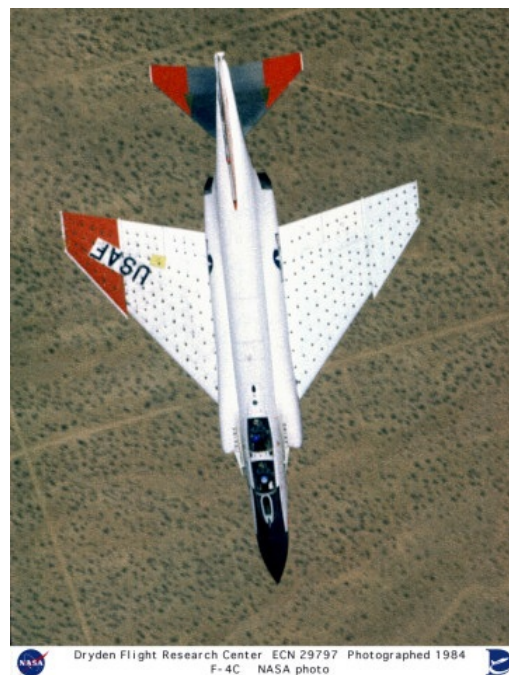
Figure 3. The F-4 Phantom II airplane at the NASA Dryden Flight Test Center, showing the flow observation tufts installed on the wings as part of the stall characteristics study. 22
