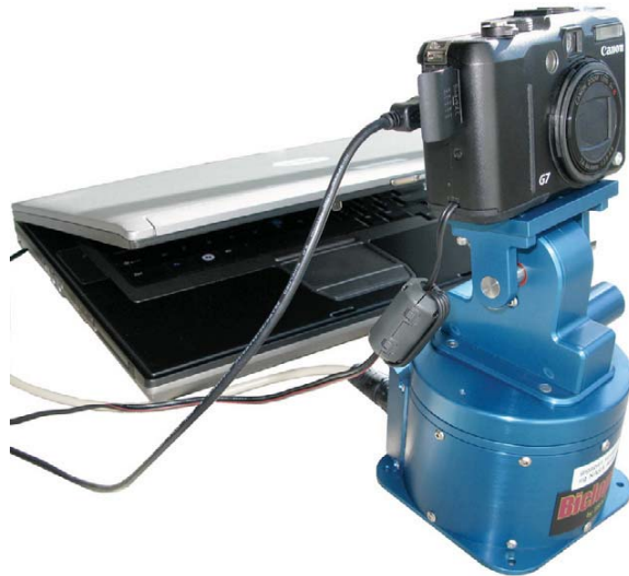
Figure 5. Gigapan Voyage is a remotely operated robotic camera for acquiring very high-resolution panoramic images.
