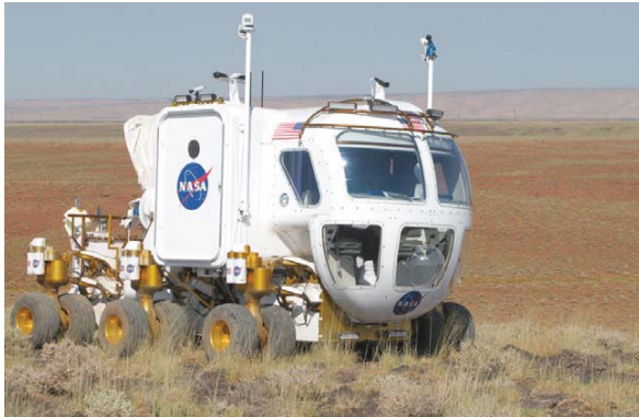
Figure 2. The Lunar Electric Rover (LER) is a prototype astronaut vehicle for planetary surface exploration during future human missions.
