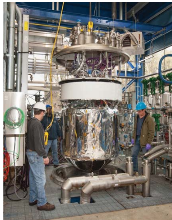
Figure 2: Liquid Hydrogen (LH 2 ) RBO Experiment Test Article Being Lowered into SMiRF Vacuum Chamber. The white ring above the test tank is the heat pipe radiator, behind which is mounted the reverse turbo-Brayton cycle cryocooler.
