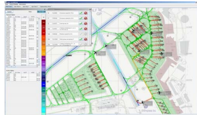
TRACC (Hamburg): a taxi route of a departure aircraft shown with speed advisories
