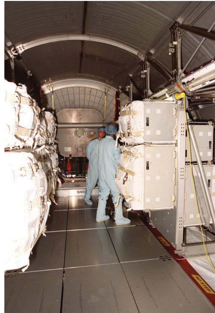
KSC-01PP-0726: Workers in the Space Station Processing Facility are removing contents from the Multi-Purpose Logistics Module (MPLM) Leonardo to begin removing the contents after STS-102. The MPLM brought back nearly a ton of trash and excess equipment from the Space Station.
