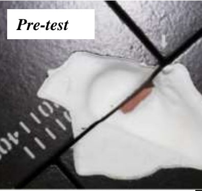
Arcjet test showed the potential for damage propagation
