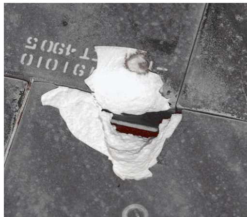
Post-flight photograph showed no damage propagation.
