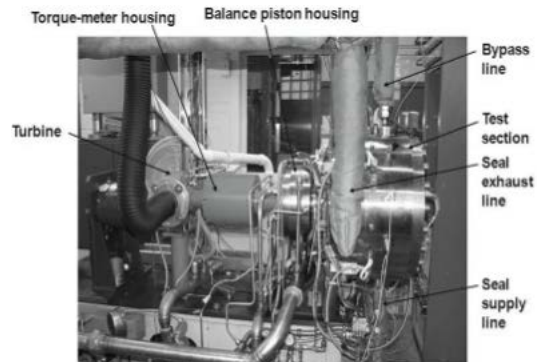
Figure 27. GRC high temperature, high speed turbine seal test facility 12 .
