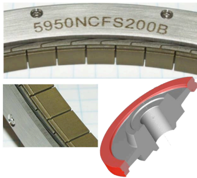
Figure 26. GRC non-contacting brush/finger turbine seal.
