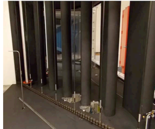
Figure 15. Photo of turbine cascade blades and rotating bar installed in USNA test facility.
